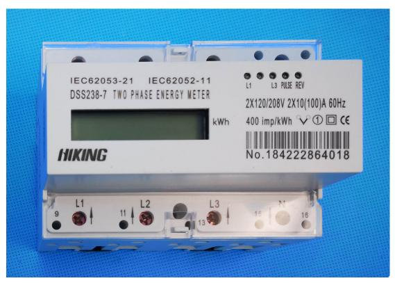
The meter is used in two phase three wire power grid. The meter is designed to measure AC active energy. All of its functions comply with the relative technical requirement for class 1 three phase watt hour meter in IEC62053-21. It is a long life meter with the advantage of high stability, high over load capability, low power loss and small volume.
